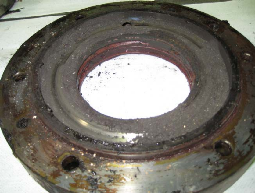
Figure 7: Photo of the bearing assembly end cap. Please note the location of the lubrication channels.
